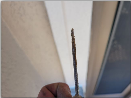
1- 1.3 Test Location K - Dark / discolored wood on probe - indication of wood rot
