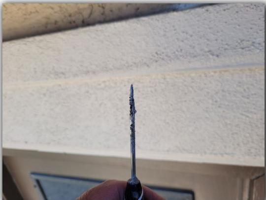
1- 1.3 Test Location K - Dark / discolored wood on probe - indication of wood rot
